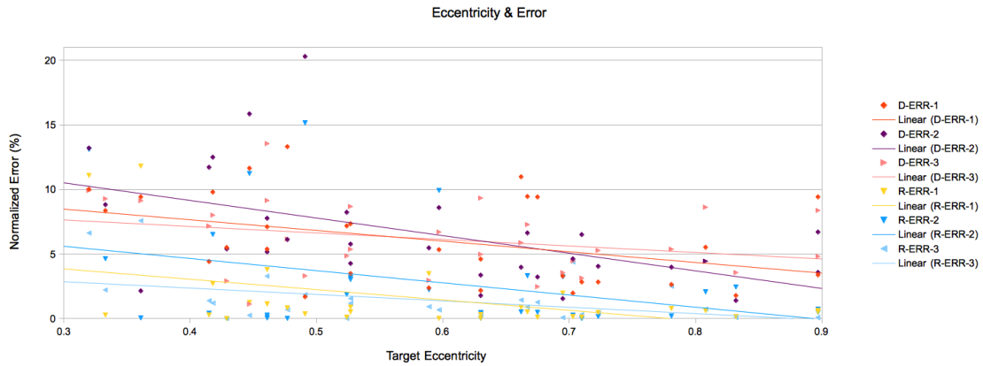
Figure 6.7: Results of normalized Distance and Rotation error (D-ERR and R-ERR respectively) recorded over successive trials as a function of target eccentricity using the gamepad controller
