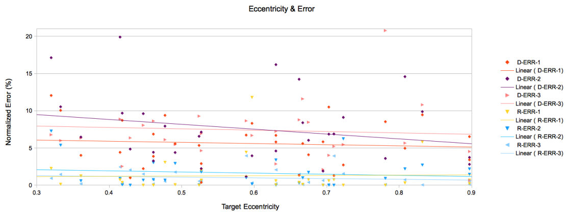
Figure 6.8: Results of normalized Distance and Rotation error (D-ERR and R-ERR respectively) recorded over successive trials as a function of target eccentricity using the LMD
